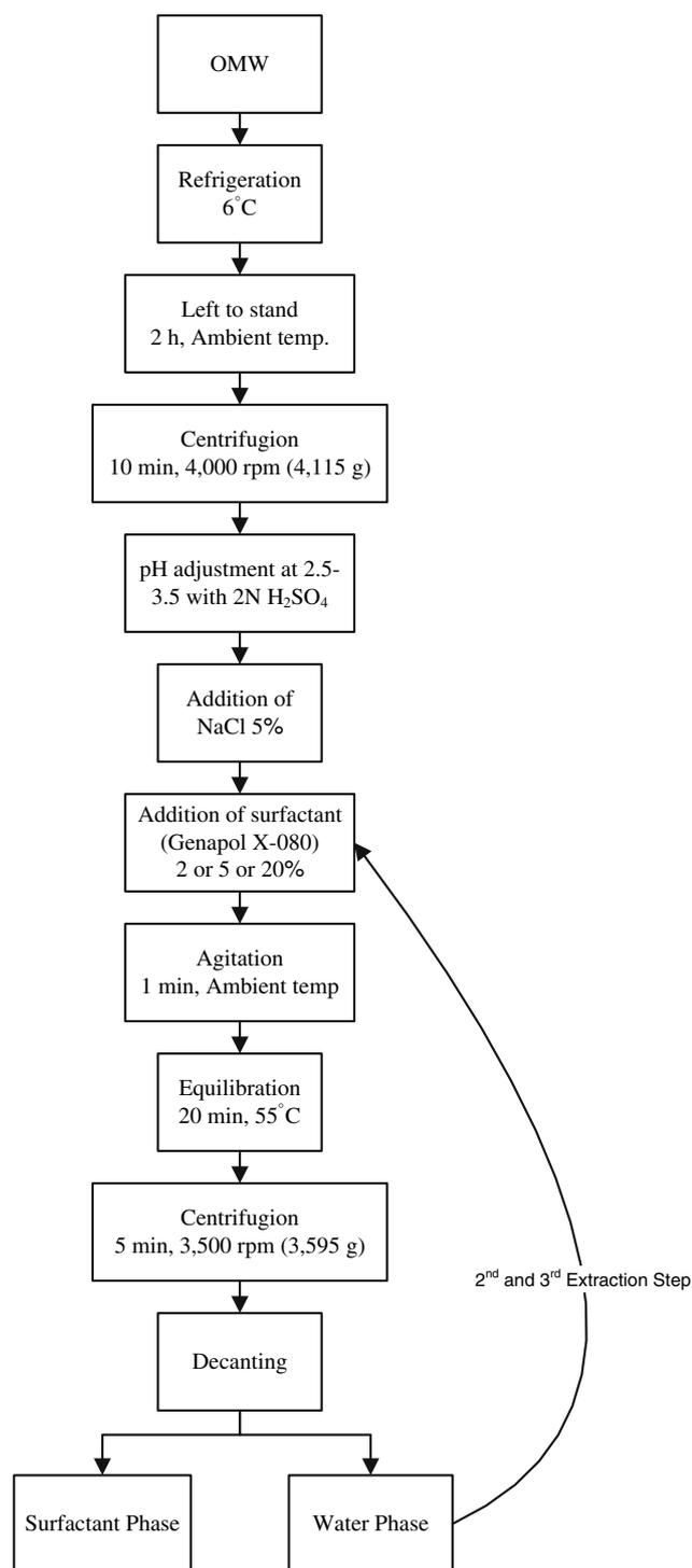
**Fig. 1** Schematic representation of the CPE procedure
